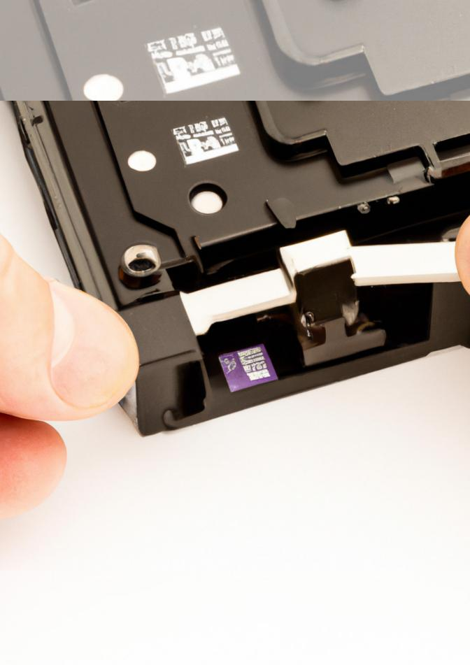
Pry the SATA connector upward while lifting the drive on your right hand to disconnect it from the logic board.
