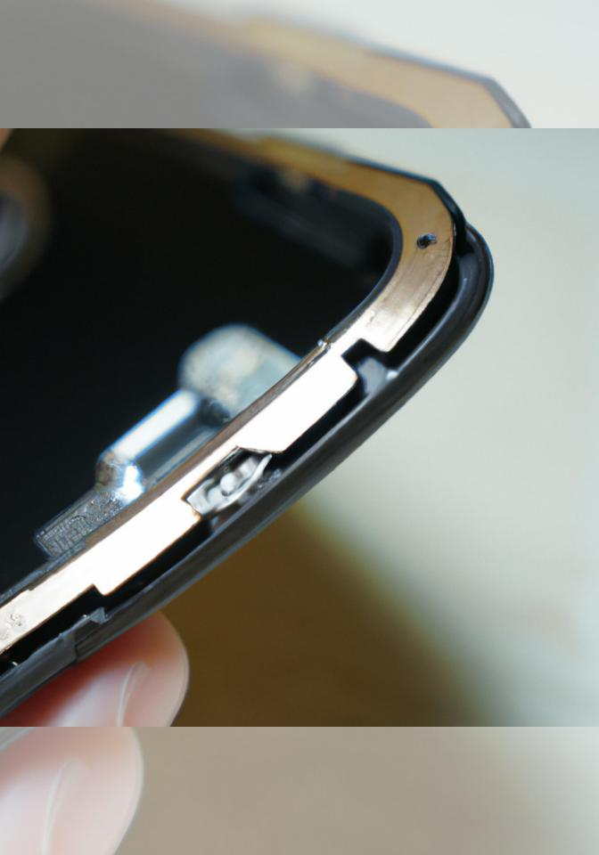
Rotate the upper case up and towards the display, so that the upper case rests against it.
