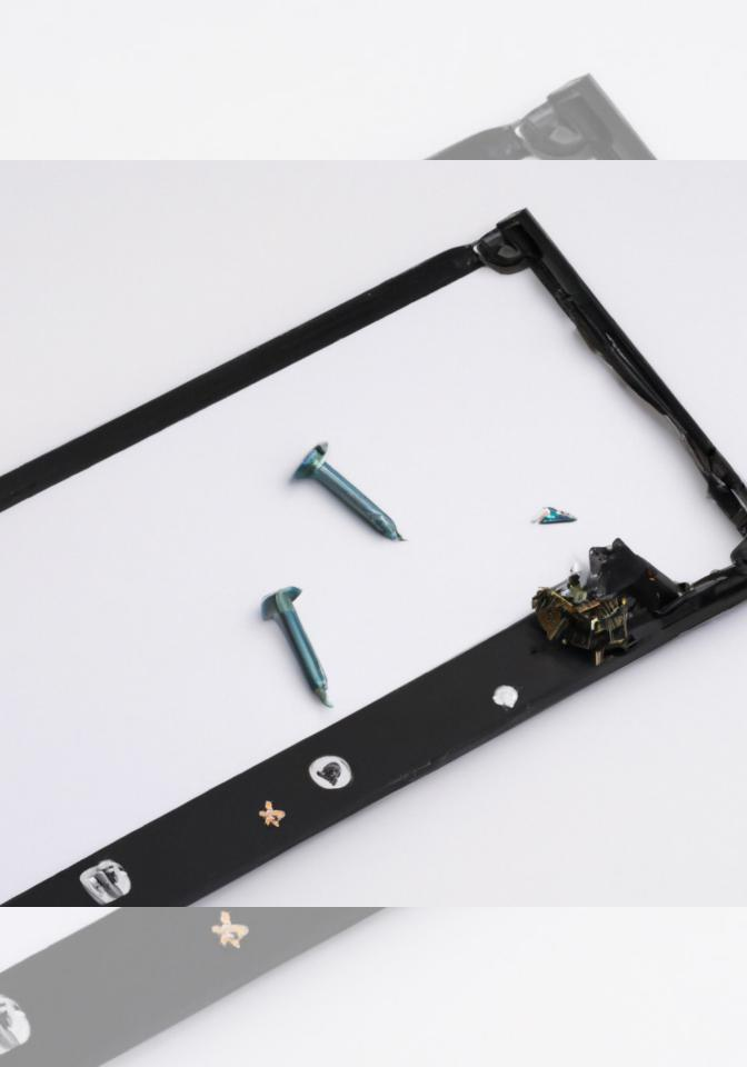
Remove the two small black Phillips screws from both sides of the display (four screws total).
