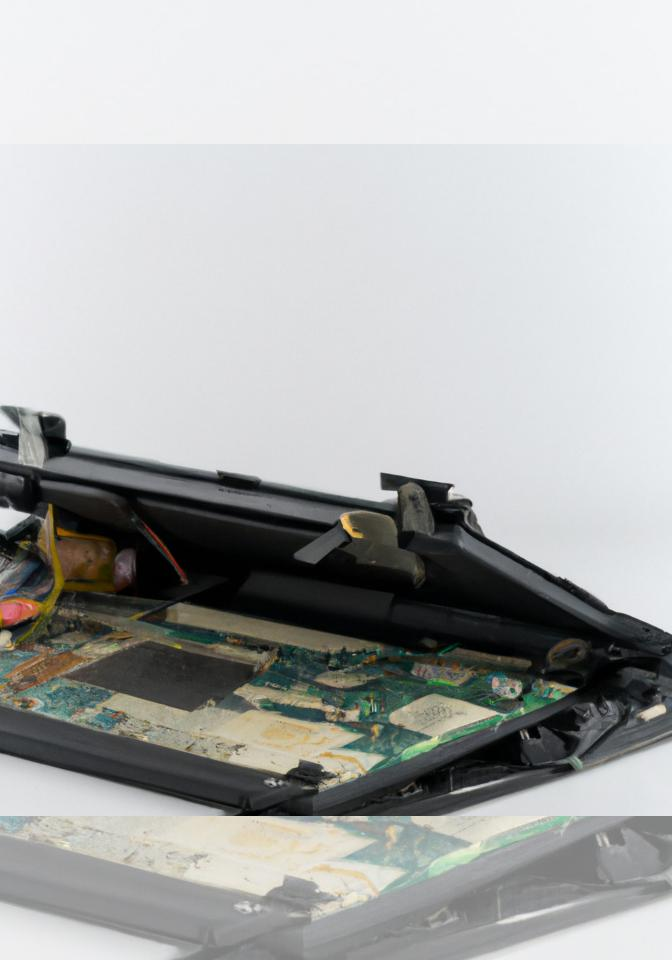
Open the computer with the display facing you and rotate the display back as far as possible.
