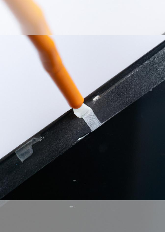
Run your spudger along the lower edge of the front display bezel to separate the adhesive from the LCD frame.
