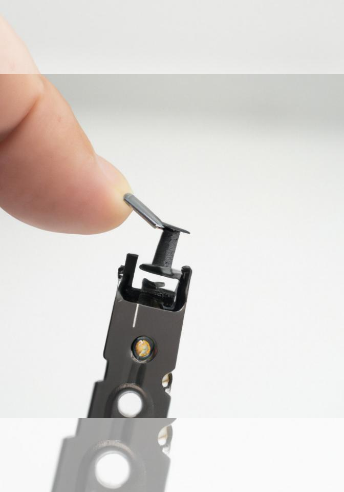
Remove the 11.5 mm T6 Torx screw Jumper from the internal metal framework by lifting it up.
