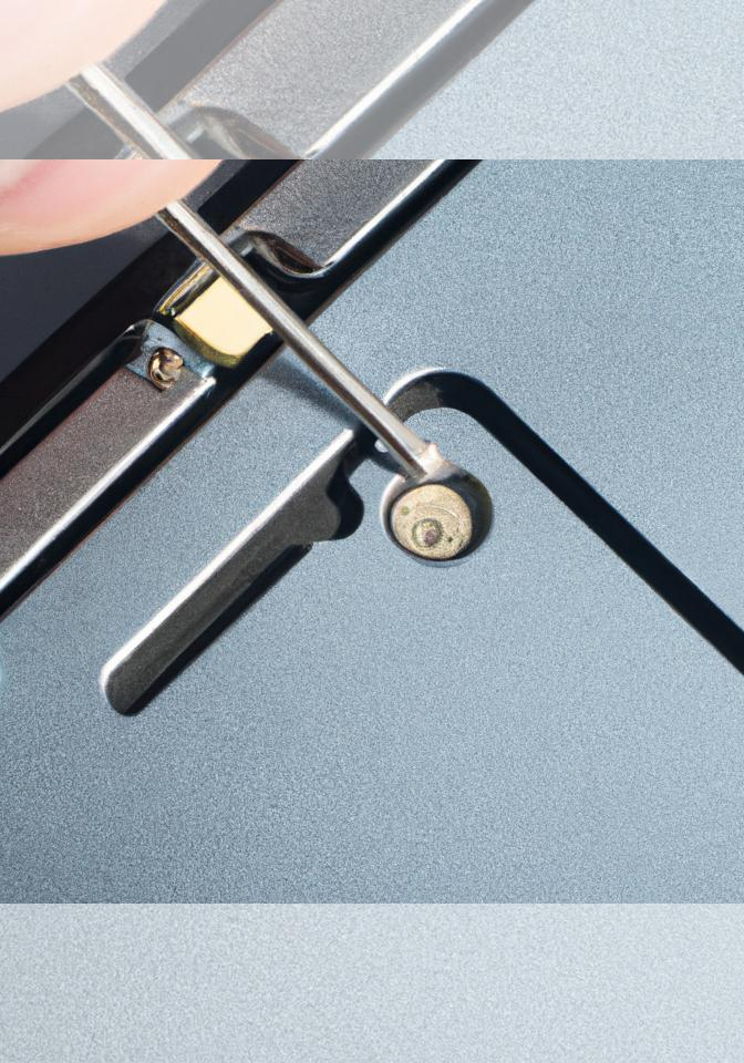
Remove the T6 Torx screw from the bottom right corner of the display assembly.
