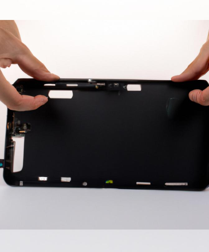
Lift the back of the case up and work your fingers along the sides, freeing the case as you go.
