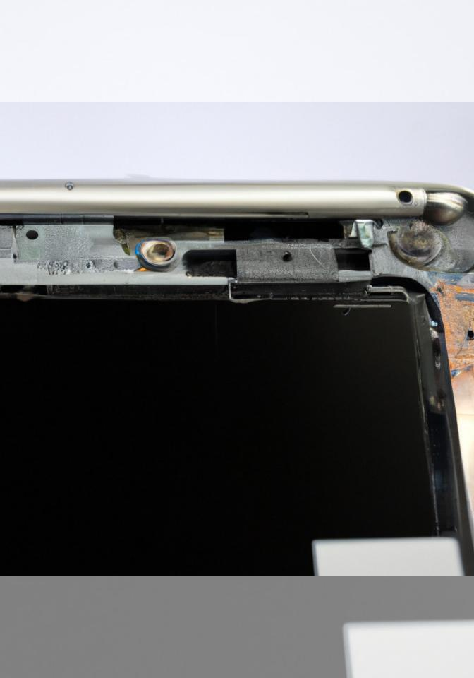
The rear bezel is still attached to the display by the antenna cables.
