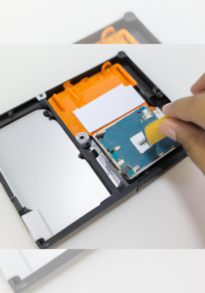
Tilt the HDD cover off the upper case.
