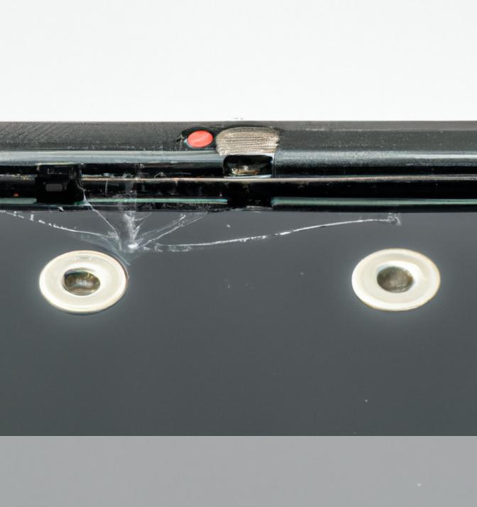
Lift the LCD off the front bezel enough to insert the flat end of a spudger between the metal LCD frame and the front display bezel.
